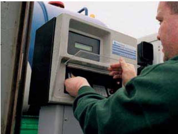
the use of the pump to authorised users only, but the data it collects is a good step towards collecting accurate data in order to run an efficient Fuel Management Programme. The information can be either printed on a small 'till roll' type printer, which is attached to the FIC, or it can be downloaded onto a microchip based module, which can be used to transfer the information to an office-based computer.
